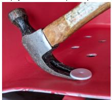
If the clips are somehow already attached to the straps, you can use the claw side of a hammer and a wrench (for extra leverage) to pry apart the clips and straps:
